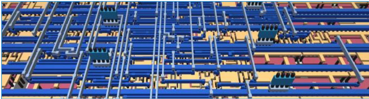
Fig. 1: Automated rendering of GDSII from the author's design [1] within the Tiny Tapeout Project
